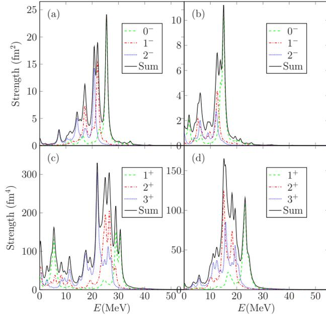
FIG. 1. Strength distributions for  $A = 76$ . (a)  $L = 1, \beta^-$ , (b)  $L = 1, \beta^+$ , (c)  $L = 2, \beta^-$ , (d)  $L = 2, \beta^+$ . The solid line denotes the sum of the dashed, dotted, and dash-dotted individual contributions. Energies are measured relative to the ground state of the odd-odd final nucleus. The strengths are given in units of  $\text{fm}^2$  for  $J^\pi = 0^-, 1^-, 2^-$  and in  $\text{fm}^4$  for  $J^\pi = 1^+, 2^+, 3^+$ .
