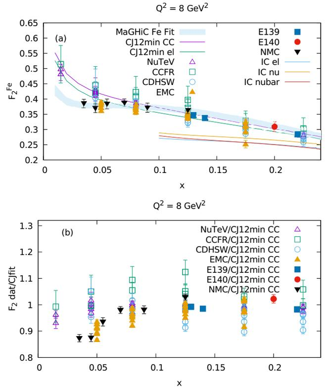
FIG. 3. (top) A low  $x$  magnification of Fig. 2 for a  $Q^2$  range of 2–20  $\text{GeV}^2$ , with (bottom) ratio data/fit, of  $F_2^{\text{Fe}}$  to the CJ12 fit for charged current neutrino vs the Bjorken scaling variable  $x$ . In both cases, the data and fits are centered to a common  $Q^2$  of 8  $\text{GeV}^2$ . Note that zero is suppressed in both plots.
