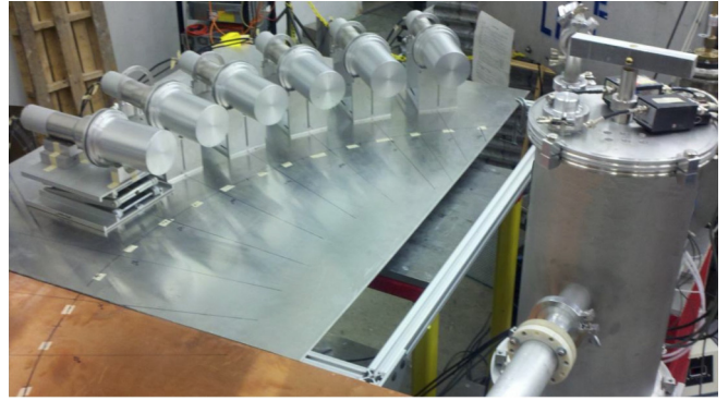
FIG. 1. The experimental setup used in the (d,n) measurements. The array of 4 \times 6 EJ315 detectors is shown positioned with the detector entrance windows 1 m from the target.
