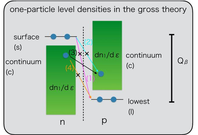
FIG. 1. One-particle level densities: (1) surface to the lowest level,  $|M_{\Omega s \rightarrow l}|^2$ ; (2) surface to continuum,  $|M_{\Omega s \rightarrow c}|^2$ ; (3) continuum to continuum,  $|M_{\Omega c \rightarrow c}|^2$ ; and (4) continuum to the lowest level,  $|M_{\Omega c \rightarrow l}|^2$ .
