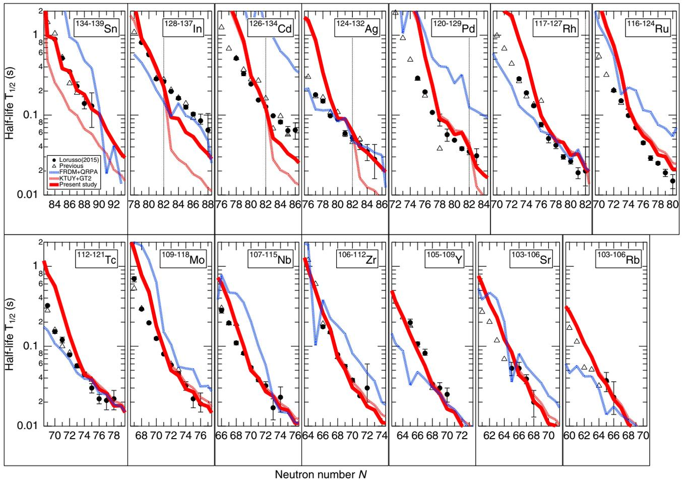
FIG. 4.  $\beta^-$ -decay half-lives for rubidium to tin isotopes in the neutron-rich mass region. Dashed red line: results of the original gross theory. Thick solid red line: results of the improved gross theory. Blue dashed line: FRDM+QRPA [12]. Open triangles: data from experiments reported prior to 2015. Solid circles: experiment results reported in 2015 [13].
