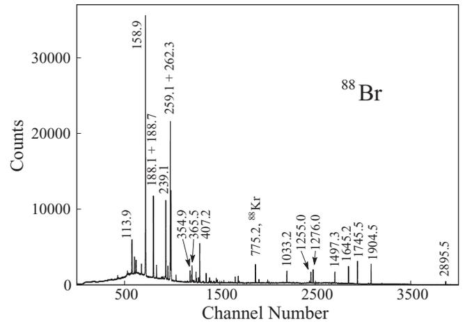
FIG. 3. A  $\beta$ -gated, singles  $\gamma$ -ray spectrum obtained in the present experiment. Energies of  $\gamma$  lines are labeled in keV. A nonlinear, constant-peak-width energy calibration was applied to enhance the low-energy part of the spectrum, where the density of lines is high.
