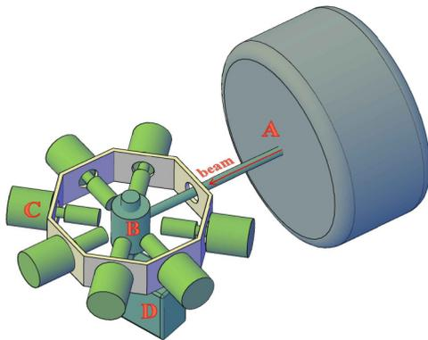
FIG. 2. Schematic view of the experimental setup. The monoisotopic ion samples released from JYFLTRAP (A) are implanted in the middle of a spectroscopic array consisting of a  $\beta$  counter (B) and seven Ge detectors (C). The moving tape collector device (D) is operating the implantation tape and removing unwanted long-lived decay products from the center of the setup.
