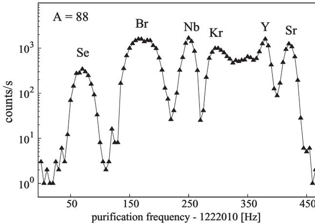
FIG. 1. Ion counts registered in the experiment using the MCP detector placed after the Penning trap. The well resolved singly charged ions from the IGISOL isobaric beam of mass  $A = 88$  are marked with their element symbol.
