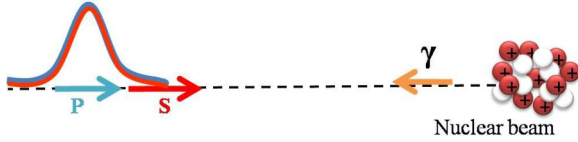
FIG. 2. Two-color scheme (copropagating beams) in the laboratory frame. The frequency of pump laser is different from that of the Stokes laser. The nuclear beam is accelerated such that \gamma(1 + \beta)\omega_{p(S)} = ck_{31(2)} is fulfilled.
