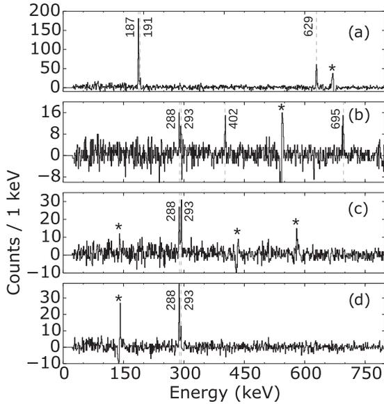
FIG. 2. Background-subtracted  $\beta$ - $\gamma$  coincidence spectra gated on the following transitions: (a) 167 keV, (b) 293 keV, (c) 402 keV, and (d) 695 keV. The peaks marked with a star ( $\star$ ) are artifacts due to the background-subtraction procedure.
