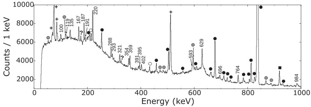
FIG. 1. Portion of the  $\beta$ -gated  $\gamma$ -ray spectrum obtained in the experiment. Transitions identified by energy were assigned to the decay of  $^{94}\text{Kr}$ . Other transitions are marked by parent decay: black circles ( $^{94}\text{Rb}$ ), gray circles (new lines assigned to decay of  $^{94}\text{Rb}$ ), open circles ( $^{94}\text{Rb } \beta n$ ), black squares ( $^{94}\text{Y}$ ), crosses for background  $\gamma$  rays, and question marks for unassigned transitions.
