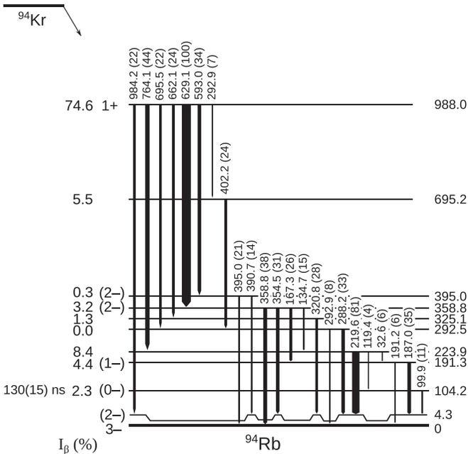
FIG. 3. Proposed  $\beta$ -decay scheme of  $^{94}\text{Kr}$ . Intensities of  $\gamma$  transitions (in brackets) are relative to the 629 keV transition. Apparent  $\beta$  feedings are calculated from  $\gamma$ -ray transitions intensities.
