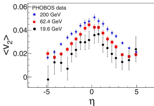
FIG. 1.  $v_2$  of charged hadrons as a function of  $\eta$  in 0-40% Au+Au collisions at  $\sqrt{s_{NN}} = 19.6, 62.4,$  and 200 GeV measured by PHOBOS experiment [7]. Only statistical errors are shown.
