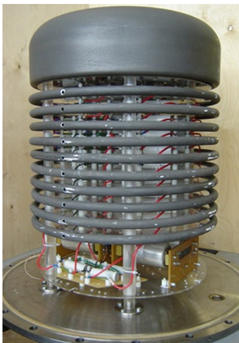
FIG. 9. (Color online) External view on the cascade multiplier.
