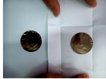
FIG. 2. (Color online) Photograph of two enriched ^{56}\text{Fe} foil samples.
