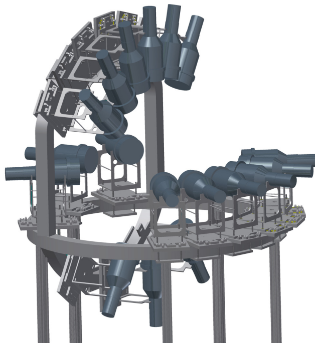
FIG. 1. (Color online) A schematic of the detector array reproduced from Ref. [1]. The detectors were located at scattering angles of \theta = 55^\circ, 72^\circ, 90^\circ, 107^\circ, 125^\circ, and 142^\circ and azimuthal angles of \phi = 0^\circ, 90^\circ, 180^\circ, 270^\circ .
