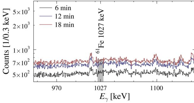
FIG. 7. (Color online) A detailed view into the region around 1027 keV of the  $\gamma$ -ray spectrum after activation with the cadmium shielding, illustrating the absence of  $^{61}\text{Fe}$  lines. Therefore, only an upper limit can be deduced from the data.
