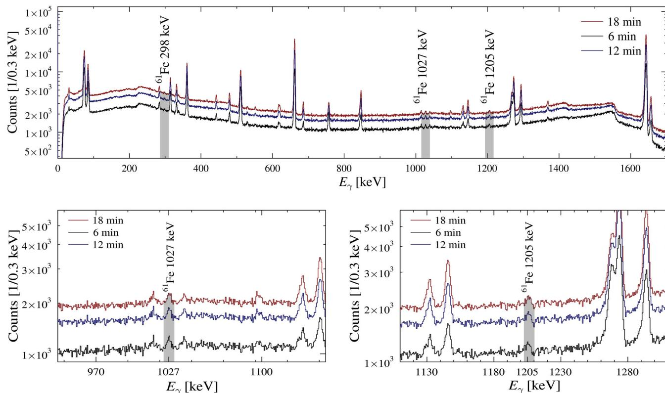
FIG. 6. (Color online) The  $\gamma$ -ray spectrum of the activation without cadmium shielding measured for one, two, and three half-lives of  $^{61}\text{Fe}$ , respectively. The upper panel provides an overview, and the lower panels show a zoom into the regions of the  $^{61}\text{Fe}$  lines at 1027 and 1205 keV. The background stems from the activation of the contaminants of the  $^{60}\text{Fe}$  sample.
