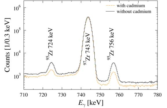
FIG. 5. (Color online) The  $\gamma$ -ray spectra of the Zr monitor foils used for the neutron fluence analysis normalized for different measuring times. Due to the smaller capture cross section of  $^{96}\text{Zr}$  in the thermal energy regime, the cadmium shielding affects the  $^{97}\text{Zr}$  signature to a much lower degree than that of  $^{95}\text{Zr}$ .
