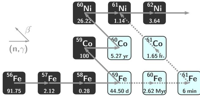
FIG. 1. (Color online) The  $s$ -process reaction path between Fe and Ni. The isotope  $^{60}\text{Fe}$  is produced via a sequence of  $(n, \gamma)$  reactions starting at the stable iron isotopes. Because of the short half-life of  $^{59}\text{Fe}$  ( $t_{1/2} \approx 45$  d), the production of  $^{60}\text{Fe}$  depends critically on the stellar neutron density.
