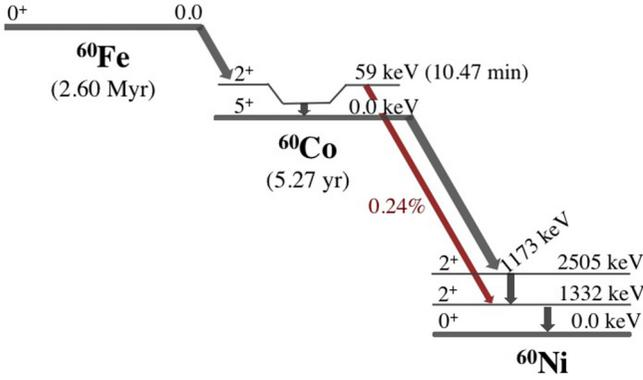
FIG. 3. (Color online) The activity of the  $^{60}\text{Fe}$  sample was determined by the  $\gamma$ -ray cascade with energies of 1173 and 1332 keV emitted after the  $\beta$  decay of the daughter nucleus  $^{60}\text{Co}$ . Data are from Refs. [17,21].
