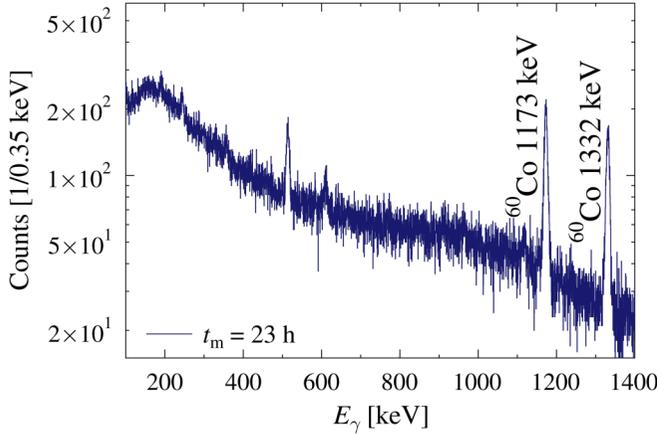
FIG. 4. (Color online)  $\gamma$ -ray spectrum for the determination of the  $^{60}\text{Co}$  activity taken 34 months after purification of the sample. The measurement time was  $t_m = 23$  h.
