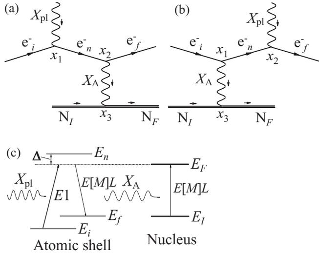
FIG. 1. Diagrams of nucleus excitation by photons through the atomic shell under the mechanism of inverse electron bridge: (a) direct diagram, (b) exchange diagram. (c) Scheme of the process corresponding to the direct diagram.
