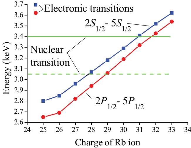
FIG. 3. (Color online) Energy of  $M1$  transitions  $5S_{1/2} \rightarrow 2S_{1/2}$  and  $5P_{1/2} \rightarrow 2P_{1/2}$  in the Rb ion shell as a function of the ion charge.
