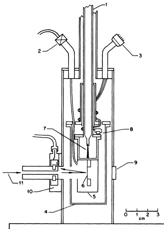
FIG. 1. Experimental arrangement for operation of the solid argon target: 1, helium transfer line; 2, inlet for argon gas; 3, electrical connections; 4, outer radiation shield; 5, inner radiation shield; 6, gold target backing; 7, needle valve for helium flow control; 8, temperature probe; 9, quartz window; 10, silicon surface barrier counter and mounting; 11, triton beam.
