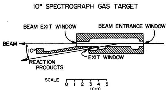
FIG. 1. Schematic view of the gas target.
