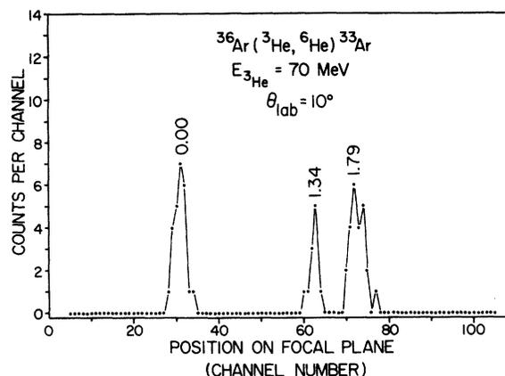
FIG. 2. Spectrum from the  $^{36}\text{Ar}(^3\text{He}, ^6\text{He})^{33}\text{Ar}$  reaction at a bombarding energy of 70 MeV and a laboratory angle of  $10^\circ$ . One channel corresponds to 43 keV in excitation.
