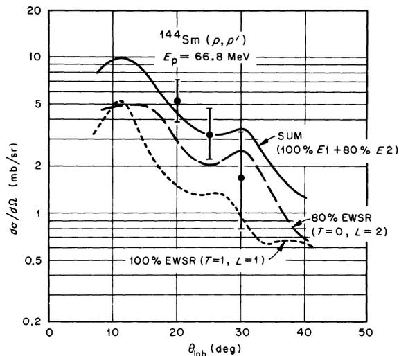
FIG. 3. Cross sections in the giant-resonance region ( $E_x \approx 10.5$ – $18$  MeV) for  $^{144}\text{Sm}$  compared to DWBA predictions. The error bars shown represent uncertainties from all sources, but are dominated by the uncertainty in the magnitude and shape of the underlying continuum.
