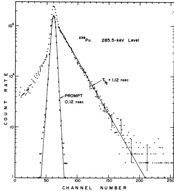
FIG. 2. The decay curve of the 285.5-keV level as measured by the 106.1-keV- $\gamma$ -277.6-keV- $\gamma$  delayed coincidence. The "prompt" curve was measured using a  $^{60}\text{Co}$  source.
