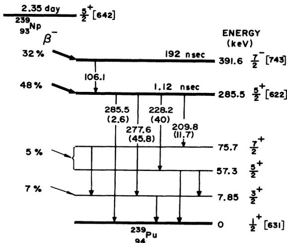
FIG. 1. Partial decay scheme of  $^{239}\text{Np}$ .
