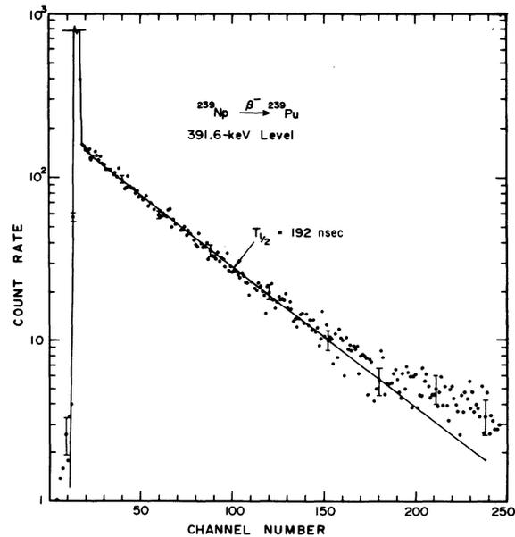
FIG. 3. The decay of the 391.6-keV level as measured by the 328-keV- $\beta$ -106.1-keV- $\gamma$  delayed coincidence.
