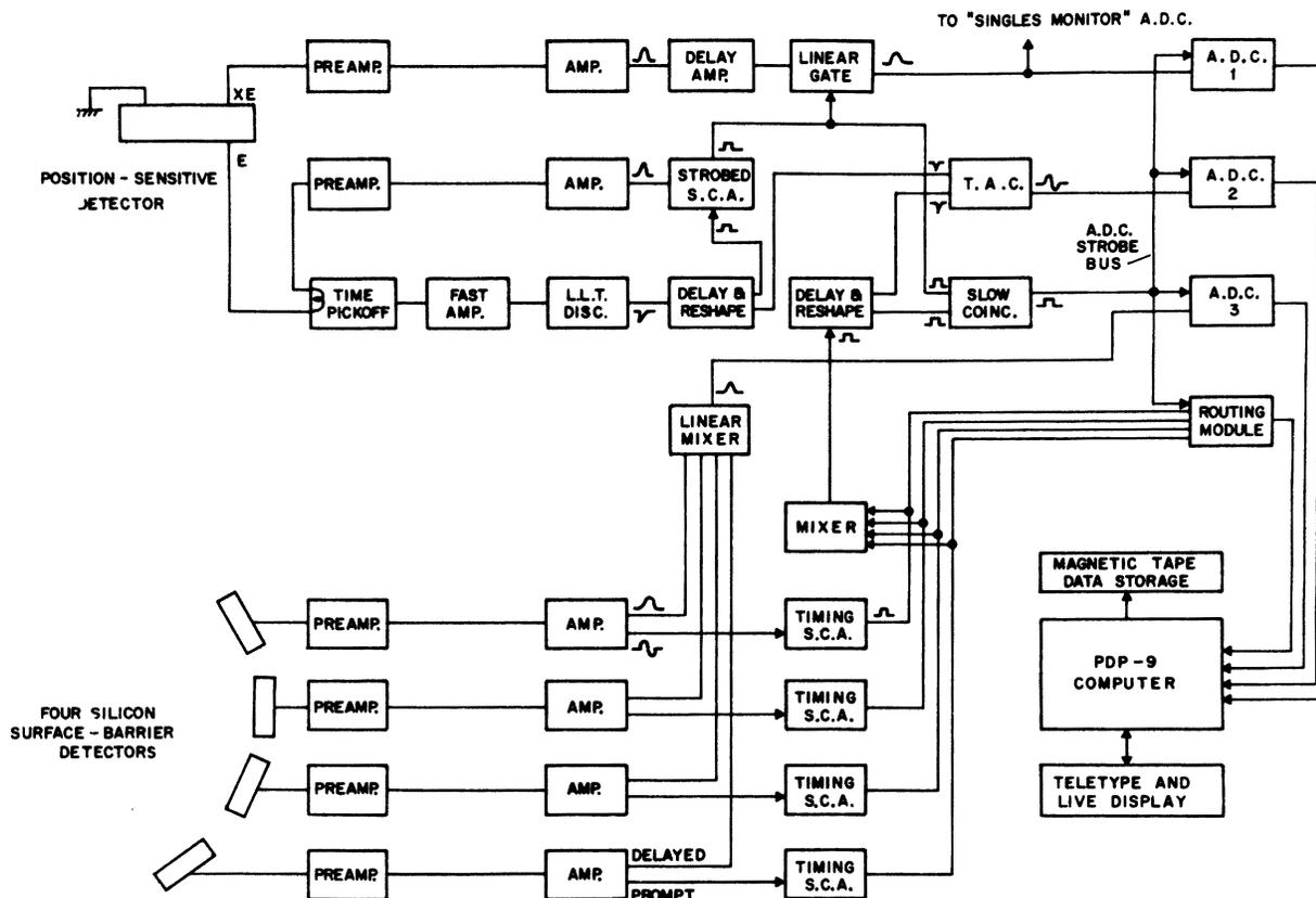
FIG. 1. Block diagram of the electronics employed for the measurements with the array of four detectors.
