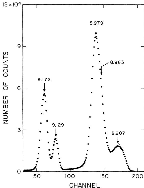
FIG. 4. Zero-degree singles proton spectrum showing the 8.91- to 9.17-MeV groups. The incident  $^3\text{He}$  energy is 12 MeV. The position-sensitive detector was placed at an angle of  $60^\circ$  to the focal plane to cover the largest practical range of excitation energy (Ref. 17). The resolution is then optimum at only one place on the detector, in this case the position corresponding to the 9.13-9.17-MeV doublet. The excitation energies are taken from Ref. 9.
