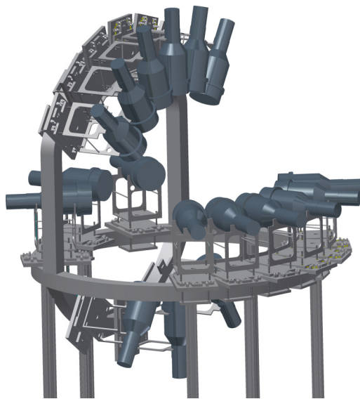
FIG. 2. (Color online) A schematic of the detector array with all eighteen detectors, reproduced from Ref. [6]. The detectors are located at scattering angles of \theta = 55^\circ, 72^\circ, 90^\circ, 107^\circ, 125^\circ , and 142^\circ .
