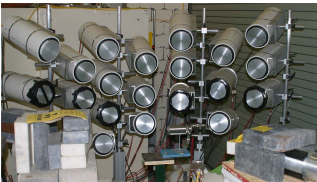
FIG. 2. (Color online) Experimental setup is as follows: FIGARO neutron detectors surrounding the fission chamber are located on seven different detection angles (45°, 60°, 75°, 90°, 105°, 112°, and 135°) with respect to the beam direction.
