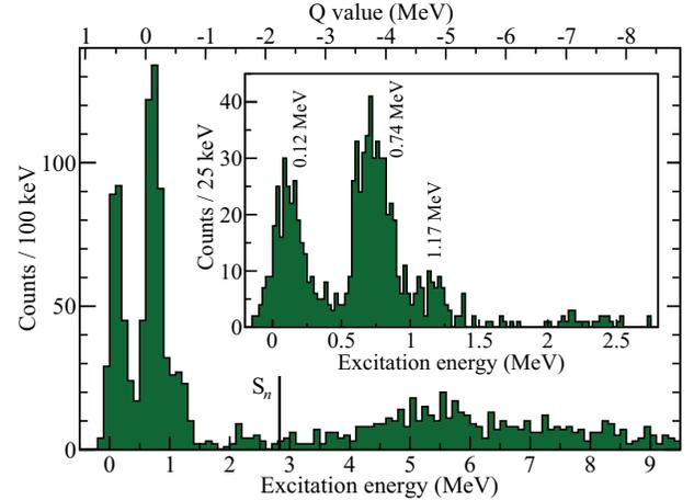
FIG. 2. (Color online) The measured excitation-energy ( $Q$ -value) spectrum for the  $^{17}\text{N}(d,p)$  reaction with the same data set as is in Fig. 1. An expanded region of the excitation energy below the neutron separation energy ( $S_n$ ) is shown in the inset.
