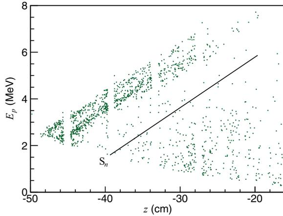
FIG. 1. (Color online) Proton energies ( $E_p$ ) as a function of the longitudinal distance from the target ( $z$ ) for the  $^{17}\text{N}(d,p)^{18}\text{N}$  reaction in inverse kinematics. The events shown required a coincidence in the recoil detector telescope with either  $^{18}\text{N}$  ions for bound states, or  $^{17}\text{N}$  for unbound ones.
