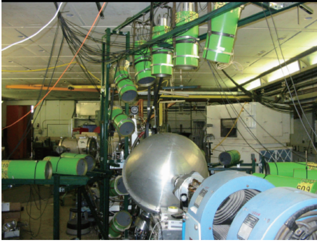
FIG. 1. (Color online) DEMON detector setup viewed from upstream of the beam. In the spherical scattering chamber, the IMF telescope and 16 CsI detectors were arranged around the target. The figure has not been digitally altered.
