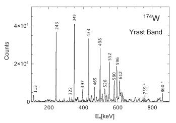
FIG. 2.  $\gamma$  spectrum obtained by gating on the lowest spin transitions of the four yrast band of <sup>174</sup>W. Energies are given for the yrast band and the strongly populated negative-parity band, labeled 4 in Ref. [14]. Stars mark interconnecting transitions.
