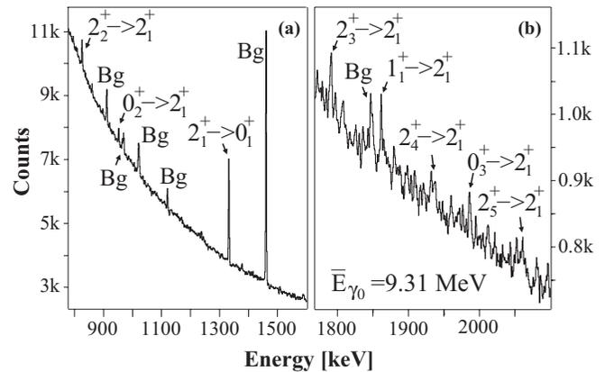
FIG. 3. Parts of a spectrum recorded perpendicular to the polarization plane. The mean energy of the incident photon beam was  $\bar{E}_{\gamma_0} = 9.31$  MeV. Peaks belonging to transitions depopulating low-lying excited states of  $^{60}\text{Ni}$  are labeled. Furthermore, peaks stemming from background transitions are labeled as BG. Please note the different scaling of the  $y$  axis.
