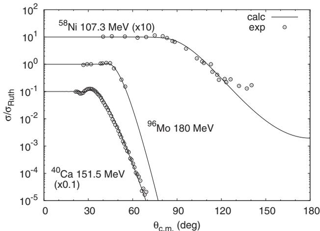
FIG. 8. Comparison between optical model calculations and experimental data for  $^{32}\text{S}$  elastic scattering from various targets at incident energies indicated in the figure. The experimental data are from Refs. [76–78].
