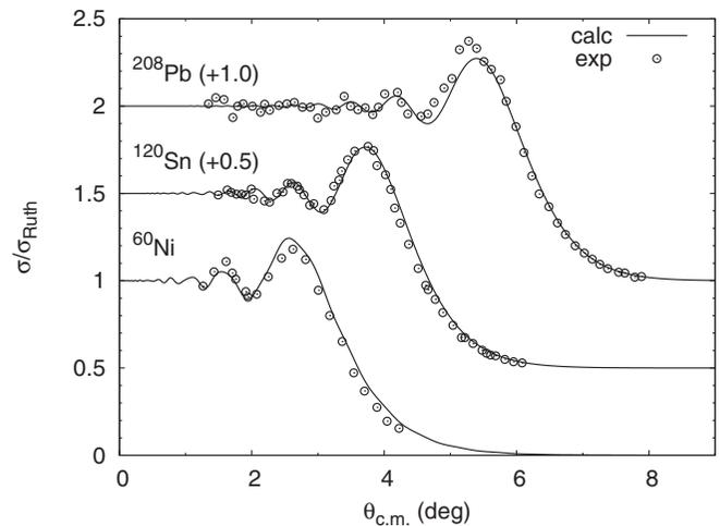
FIG. 9. Comparison between optical model calculations and experimental data for  $^{40}\text{Ar}$  elastic scattering from  $^{60}\text{Ni}$ ,  $^{120}\text{Sn}$ , and  $^{208}\text{Pb}$  at 44 MeV/nucleon. The experimental data are from Ref. [79].
