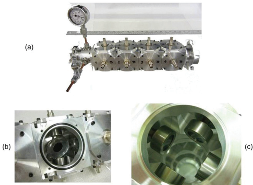
FIG. 5. (Color online) Photographs of cubical scattering chamber array showing (a) overall view, (b) the target and detectors, and (c) the detectors only.
