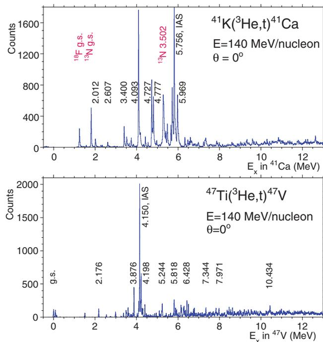
FIG. 8. (Color online) Comparison of (a) the  $^{41}\text{K}(^3\text{He},t)^{41}\text{Ca}$  spectrum and (b) the  $^{47}\text{Ti}(^3\text{He},t)^{47}\text{V}$  spectrum measured at 140 MeV/nucleon and  $0^\circ$ . The scales of the ordinates are adjusted so that the states with the same  $B(\text{GT})$  value have the same height in these two spectra.
