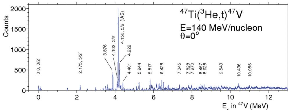
FIG. 1. (Color online) The  $^{47}\text{Ti}(^3\text{He}, t)^{47}\text{V}$  spectrum at  $0^\circ$ . Events with scattering angles  $\Theta \leq 0.5^\circ$  are included. Prominent states populated in  $\Delta L = 0$  transitions are indicated by their excitation energies.
