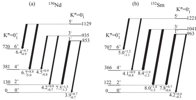
FIG. 1. Comparison of  $B(E1)$  values (in  $\text{mW.u.} = 10^{-3} \text{ W.u.}$ ) for the transitions between the levels of the  $K^\pi = 0^-$  and  $K^\pi = 0^+$  bands of (a)  $^{150}\text{Nd}$  and (b)  $^{152}\text{Sm}$ . The widths of the arrows are proportional to the central  $B(E1)$  values of the corresponding transitions. The  $B(E1)$  values with the associated uncertainties for the corresponding decays are shown at the bottom of the transition arrows.
