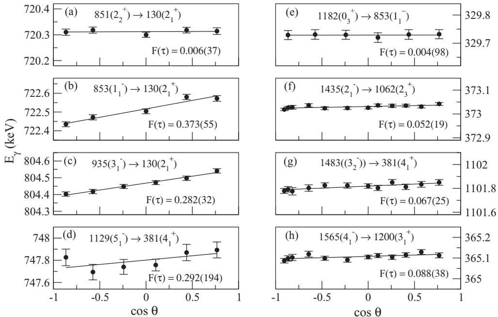
FIG. 6. The measured energies as a function of  $\cos\theta$  for  $\gamma$  rays from several levels of interest. The data presented are from the angular distribution measurements at  $E_n = 1.2$  [(a), (b)], 1.4 [(c)–(e)], and 2.05 [(f)–(h)] MeV. Linear fits to the data are shown, and the corresponding  $F(\tau)$  values are indicated. The lifetimes of the levels are extracted from these data (see Table I and text for details).
