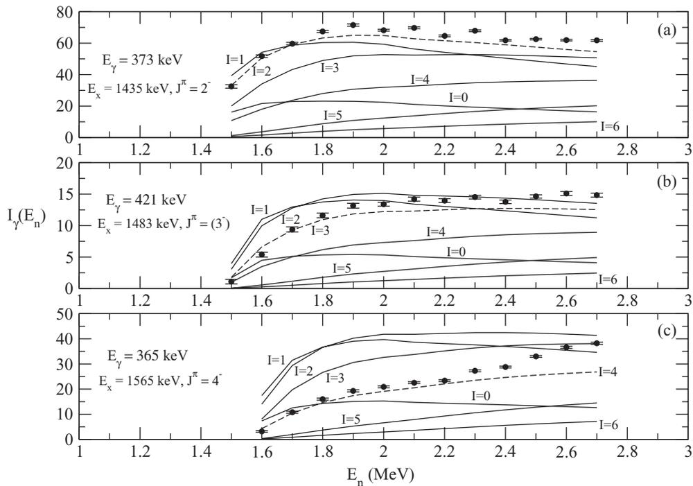
FIG. 4. The excitation function curves of (a) 373-, (b) 421-, and (c) 365-keV  $\gamma$  rays from the 1435-, 1483-, and 1565-keV levels, respectively [cf. Fig. 2(a)]. The experimental results are compared with calculations from the code CINDY [24] for possible spins of the levels with negative parities. The theoretical calculations giving the best fits to the experimental data are shown as dashed lines. The theoretical curves do not include feeding from higher-lying states.
