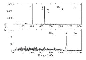
FIG. 3. (a) Singles  $\gamma$ -ray spectrum in one clover segment showing the transitions in <sup>126</sup>Te arising from the decay of the contaminant <sup>126</sup>Sb in the beam. (b) All the  $\gamma$  rays in coincidence with particles selected in all solar cells for both backward clover detectors. The randoms subtraction eliminated effectively all  $\gamma$  lines stemming from the radioactive beam contamination.
