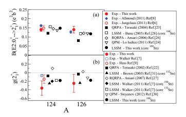
FIG. 5. (Color online) A compilation of calculated  $B(E2:0^+_1 \rightarrow 2^+_1)$  (a) and  $g(2^+_1)$  (b) values including the experimental data (points with error bars) for <sup>124</sup>Sn and <sup>126</sup>Sn. The core (<sup>100</sup>Sn or <sup>132</sup>Sn) used in each LSSM calculation is indicated in the legend.
