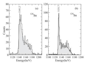
FIG. 4. Line-shape fits of the  $(2_1^+ \rightarrow 0_1^+)$  transition in <sup>126</sup>Sn (a) and <sup>124</sup>Sn (b) at a detector angle of 59°. The broad stopped peak in <sup>126</sup>Sn is due to decay in a gap between the multilayer target and attached stopper foil (see text).
