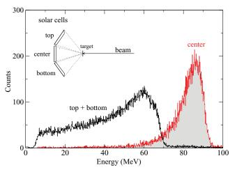
FIG. 2. (Color online) Spectra observed in the central and adjoining solar cells.
