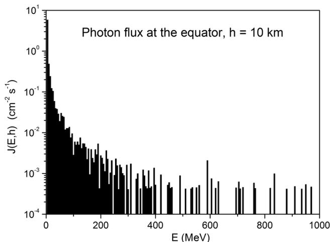
FIG. 3. Calculated equatorial  $\gamma$ -ray flux at the altitude of 10 km in the Earth’s atmosphere at moderate solar activity.
