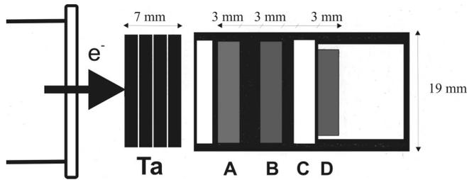
FIG. 1. Layout of the target irradiation on the accelerator. “Ta” denotes the four tantalum plates converter; A and B denote the Al containers with powdered nitrides AlN and BN, respectively; C denotes the corundum target ( $\text{Al}_2\text{O}_3$ ), and D denotes the carbon target.
