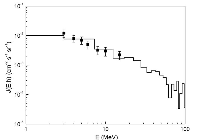
FIG. 4. Results of the calculation of the  $\gamma$ -ray flux at moderate solar activity at the altitude of 5 km in the terrestrial atmosphere (solid line) at temperate latitudes. Squares are the experimental data from Ref. [13].
