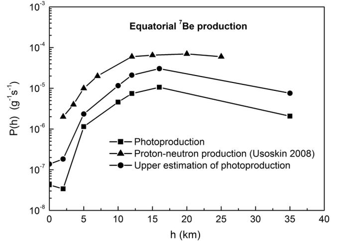
FIG. 5. Results of the numerical calculation of the rate of the photoproduction of  ${}^7\text{Be}$  as a function of the altitude in the equatorial region. The contribution of the proton-neutron mechanism is shown for comparison (Ref. [3]).
