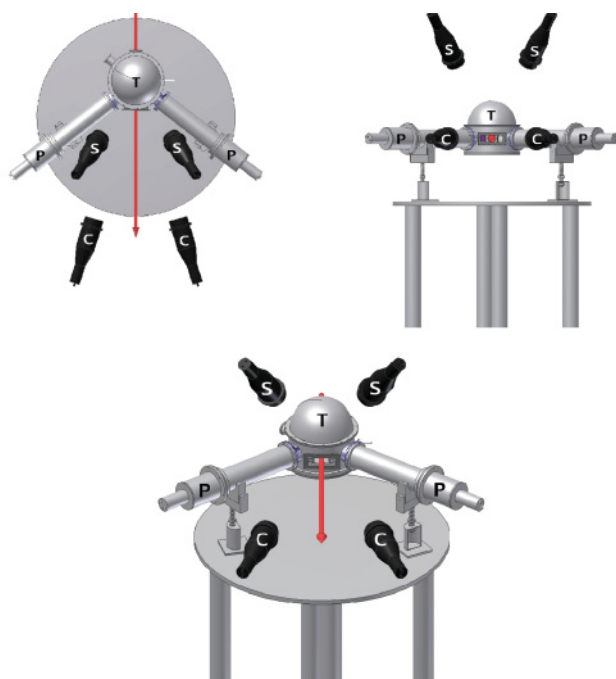
FIG. 2. (Color online) Three-dimensional renderings of top, front, and perspective views of experimental setup showing the target chamber (T), the charged particle arms (P), the SST (S) and CST (C) neutron detectors, and the neutron beam (red arrow). Please note that, in the front view, the neutron beam direction is out of the page.
