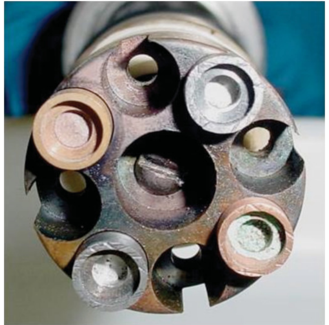
FIG. 1. (Color online) Photograph of the ion-source cathode assembly for the second production run. Four cathodes are filled beginning clockwise from the upper-right position: ^{nat}\text{Sr} in Ag, ^{nat}\text{Sr} in Cu, ^{82}\text{Sr} in Ag, and ^{nat}\text{SrO} in Cu. The cathodes with Ag are in Ta cups and the others are in Cu holders. The first three cathodes were produced using the same technique. The fourth was produced by mixing \text{SrO} powder with Cu powder before filling and pressing.
