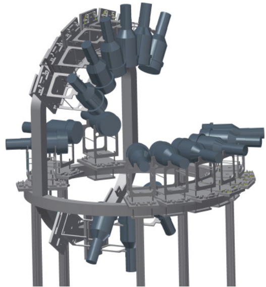
FIG. 2. (Color online) A schematic of the half-meter flight-path detector array.
