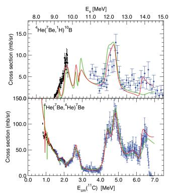
FIG. 3. (Color online) Measured cross sections for the  ${}^4\mathrm{He}({}^7\mathrm{Be},\,p){}^{10}\mathrm{B}$  (top) and  ${}^4\mathrm{He}({}^7\mathrm{Be},\,\alpha){}^7\mathrm{Be}$  (bottom) reactions. The red lines show the *R*-matrix fit to the data with  $R_0=1.4$  fm. Blue data points indicate the high-energy data measured at ORNL and the black data points are the data from LLN. The error bars indicate statistical errors only. The green line shows the *R*-matrix fit with  $R_0=1.3$  fm.
