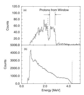
FIG. 2. (a) Proton and (b)  $\alpha$ -particle laboratory energy spectra from the  $E(^7\text{Be}) = 7.1\text{-MeV}$  data. The vertical dashed lines indicate the maximum energy protons and  $\alpha$  particles expected from the resonant scattering reactions. In part (a) the region of the spectrum corresponding to protons knocked out of the Mylar window foil is indicated.
