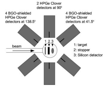
FIG. 2. A schematic view of the setup. In the center the target chamber is shown with target and stopper foil and the Si detector at  $0^{\circ}$ . The chamber is surrounded by ten clover detectors. The beam is coming from the left.
