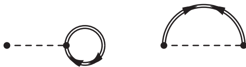
FIG. 1. First-order normal \Sigma^{11(1)} (left) and anomalous \Sigma^{21(1)} (right) self-energy diagrams. Double lines denote self-consistent normal (two arrows in the same direction) and anomalous (two arrows in opposite directions) propagators while dashed lines embody antisymmetrized matrix elements of the NN interaction.
