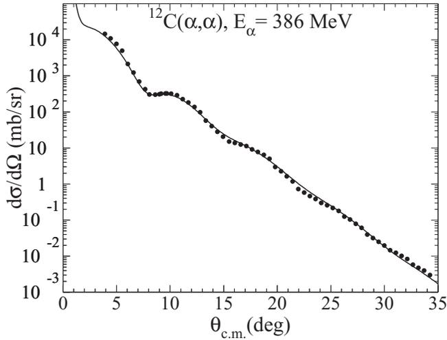
FIG. 2. Angular distribution of elastic scattering from  $^{12}\text{C}$  at  $E_\alpha = 386$  MeV. The solid line shows the result of the DWBA calculation using the single-folding model with the effective  $N\text{-}\alpha$  interaction.
