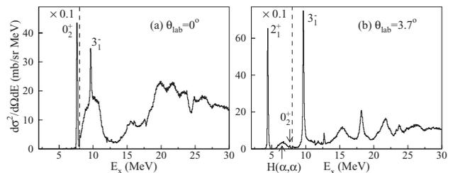
FIG. 1. Energy spectra for the  $^{12}\text{C}(\alpha, \alpha')$  reaction at scattering angles (a)  $\theta_{\text{lab}} = 0^\circ$  and (b)  $\theta_{\text{lab}} = 3.7^\circ$ . The momentum acceptances of the spectrometer were in the range of  $3 \leq E_x \leq 30$  MeV at  $2.0^\circ$ – $15^\circ$  and of  $7 \leq E_x \leq 30$  MeV at  $0^\circ$ , respectively.
