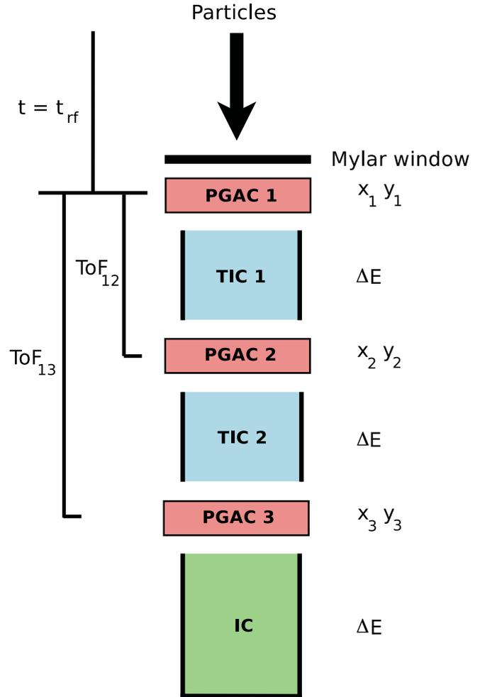
FIG. 2. (Color online) Focal plane detection system used in the present study [18]. Residues are rigorously discriminated through a set of multiple PGACs and ion chambers. The time-of-flight parameters used in the analysis are indicated.
