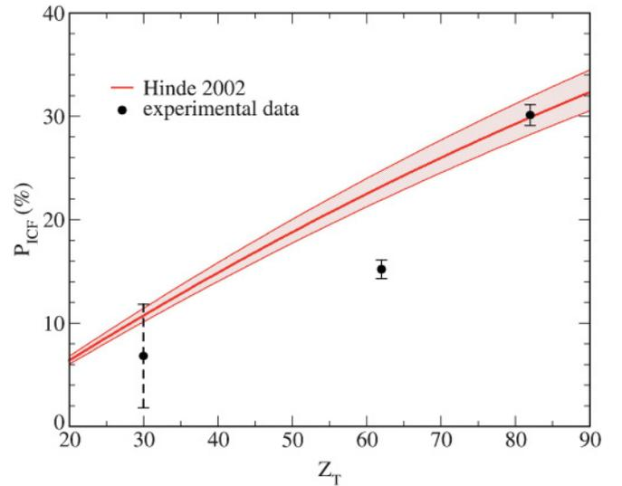
FIG. 2. (Color online) Mean experimental probability of incomplete fusion at energies slightly above the Coulomb barrier, for the two systems for which it is available. The dashed point is an estimation of  $P_{\text{ICF}}$  for the  $^{64}\text{Zn}$  target [12]. The shaded band is an empirical prediction by Hinde [23] for this value.
