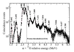
FIG. 1. (Color online)  $\alpha + {}^{15}\text{O}$  coincidences versus relative energy in  ${}^{19}\text{Ne}$ . The shaded circles are experimental data while the red curves are the fit. Excitation energies in MeV are indicated.
