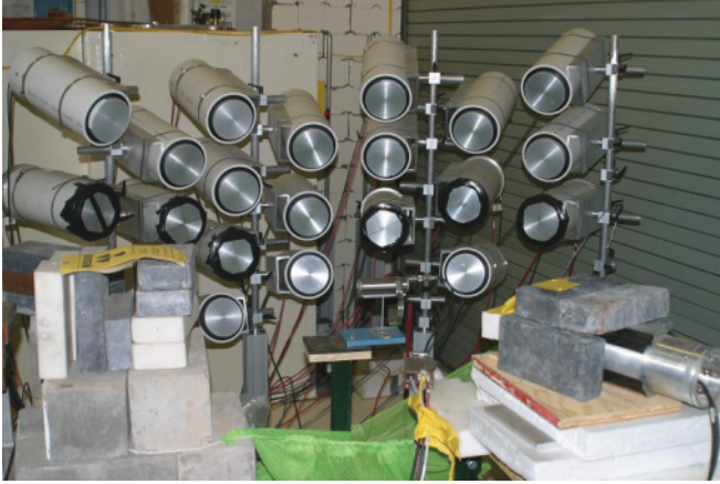
FIG. 3. (Color online) The FIGARO array, consisting of 20 EJ301 neutron detectors and a BaF 2 \gamma -ray detector.
