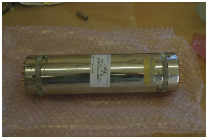
FIG. 2. (Color online) The CEA fission chamber, showing the overall appearance.
