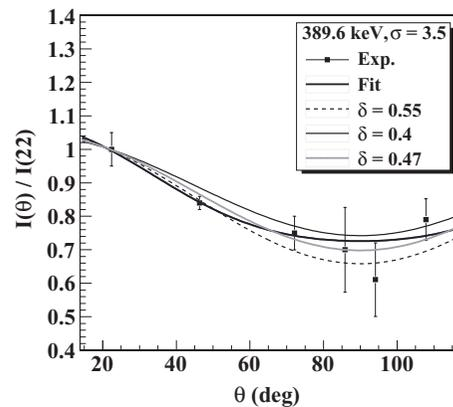
FIG. 5. Angular distributions for the 389.6 keV ( $8^- \rightarrow 7^-$ ) transition. The fit of the experimental points is shown by the black curve. With  $\sigma = 3.5$  the data are well reproduced by the theoretical curve using  $\delta = 0.47$  (gray). Dot-dashed ( $\delta = 0.40$ ) and dashed ( $\delta = 0.55$ ) curves illustrate the sensitivity of the method to the  $\delta$  parameter.
