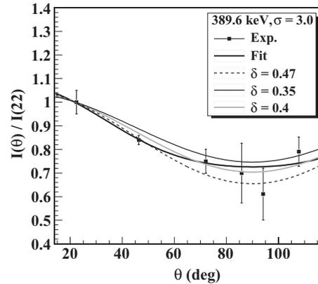
FIG. 4. Angular distributions for the 389.6 keV ( $8^- \rightarrow 7^-$ ) transition. The fit of the experimental points is shown by the black curve. With  $\sigma = 3.0$  the data are well reproduced by the theoretical curve using  $\delta = 0.4$  (gray). Dot-dashed ( $\delta = 0.35$ ) and dashed ( $\delta = 0.47$ ) curves illustrate the sensitivity of the method to the  $\delta$  parameter.
