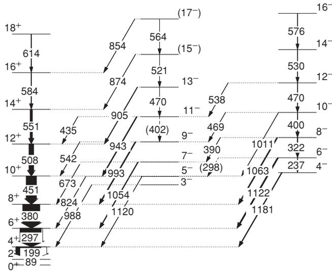
FIG. 1. Partial level scheme of  $^{156}\text{Gd}$ , established in this work, showing the ground-state band, odd- and even-spin negative-parity bands, as well as the linking transitions.
