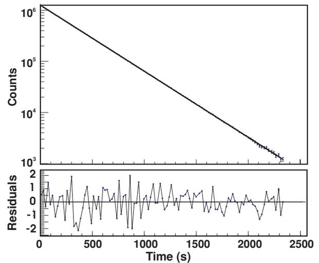
FIG. 1. (Color online) The decay of  $^{198}\text{Au}$  in gold (III) oxide, at room temperature. Experimental data appear as dots in the upper portion of the figure; the straight line is the fit to these data. Normalized residuals are shown at the bottom.
