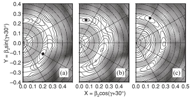
FIG. 5. Potential-Energy Surface (PES) calculations for  $^{112}\text{Tc}$  for a negative-parity neutron and a positive-parity proton ( $-\nu, +\pi$ ) (a),  $+\nu, +\pi$  (b), and  $-\nu, -\pi$  (c). Isolines are placed at intervals of 200 keV and the energies of the minima in (b) and (c) are 411 and 474 keV relative to the  $-\nu, +\pi$  ground state. The  $+\nu, -\pi$  configuration is also calculated to be triaxial but at an even higher excitation energy.
