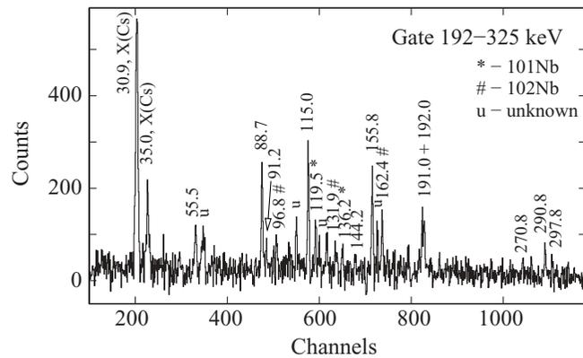
FIG. 2. LEPS spectrum double gated on the 192- and 325-keV  $\gamma$  lines of  $^{145}\text{Cs}$ . Energies are labeled in keV. See text for further explanations.
