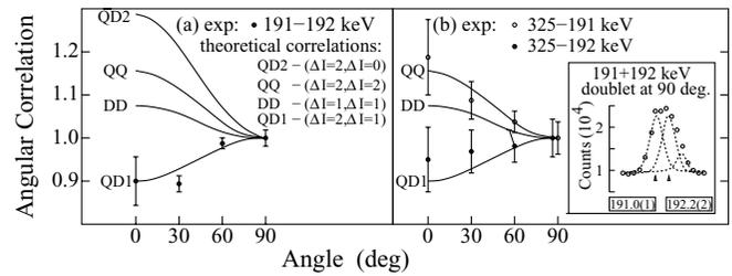
FIG. 6. Angular correlations between the 191.0-, 192.0-, and 325.3-keV lines of  $^{145}\text{Cs}$ , as observed in this work. Theoretical correlations are for unmixed transitions. See text for further explanations.
