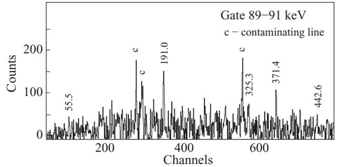
FIG. 3. A  $\gamma$ -ray spectrum double gated on 88.7- and 91.0-keV lines in  $^{145}\text{Cs}$ . Lines are labeled in keV. See the text for further explanations.
