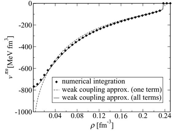
FIG. 1. Neutron pairing strength  $v^{\pi n}[\rho_n, \rho_p]$ , as defined by Eq. (3), vs nucleon number density  $\rho$  in symmetric nuclear matter using the effective interaction underlying the nuclear mass model HFB-17 [12,13]. The symbols are the results of numerically integrating Eq. (4). The dashed and solid lines were obtained using Eqs. (9) (12), respectively.
