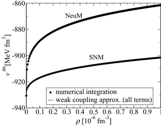
FIG. 3. Neutron pairing strength  $v^{\pi n}[\rho_n, \rho_p]$ , as defined by Eq. (3), vs nucleon number density  $\rho$  in symmetric nuclear matter (SNM) and pure neutron matter (NeuM) using the effective interaction underlying the nuclear mass model HFB-17 [12,13]. The symbols are the results of numerically integrating Eq. (4) and the solid line was obtained from Eq. (12).
