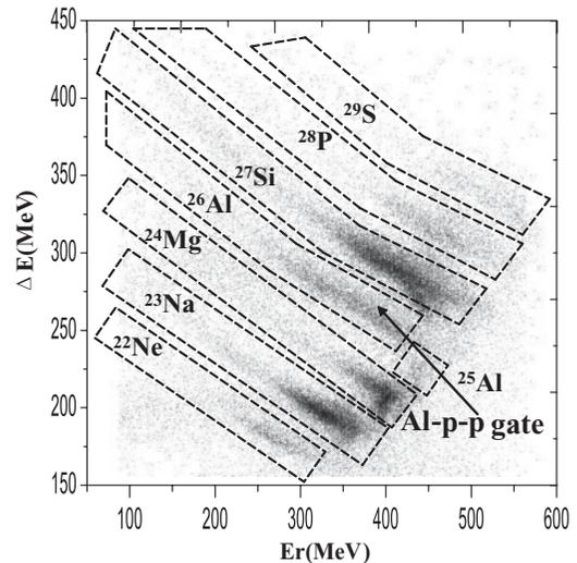
FIG. 3. Two-dimensional matrix for identification of heavy fragments after the target. The energy loss in SSSD1 ( $\Delta E$ ) is plotted versus the sum of the residual energy loss ( $E_r$ ) in SSSD2 and SD2.
