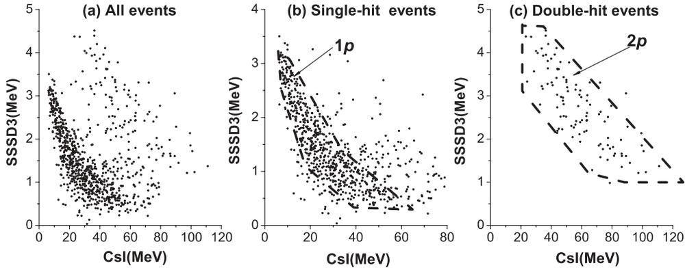
FIG. 4. Light particle identification spectrum from the detector array. Energy loss in SSSD3 is plotted as a function of the residual energy in the CsI + PIN detector array. In the construction of  $2p$  emission from  $^{28}\text{P}$  excited levels, a  $2p$  gate for Al- $p$ - $p$  coincidence was selected.
