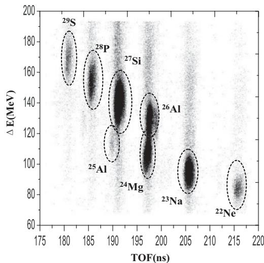
FIG. 2. Particle identification spectrum of energy loss from SD1 versus time of flight between the two plastic scintillators for RIBs.
