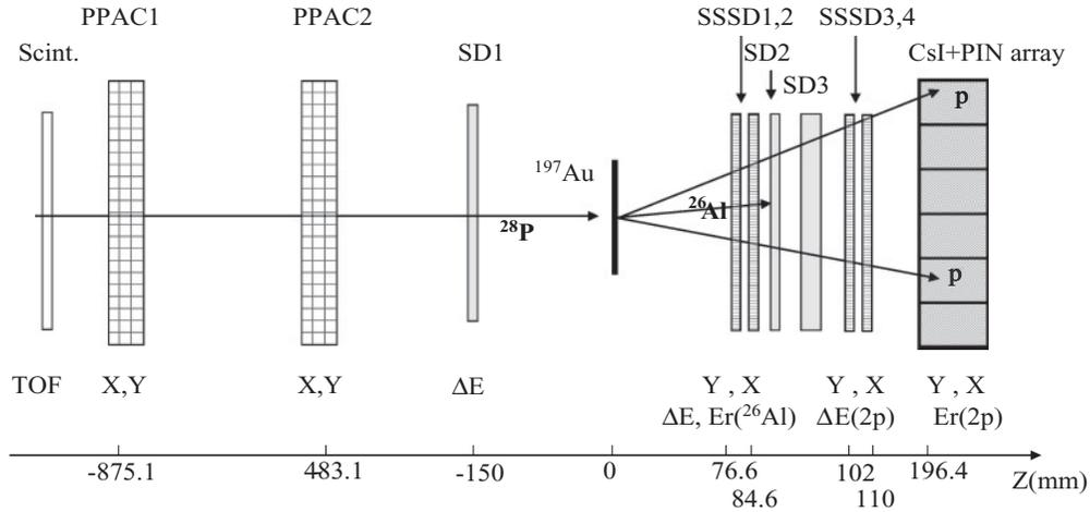
FIG. 1. Schematic of the detection setup designed for the study of exotic emission of  $^{28}\text{P}$  by complete-kinematics measurement.
