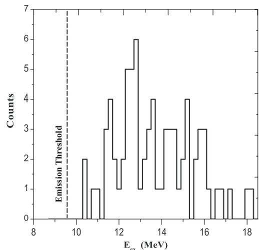
FIG. 5. Reconstructed excited energy spectrum for  $^{28}\text{P}$  from three-body correlations of Al- $p$ - $p$  events.
