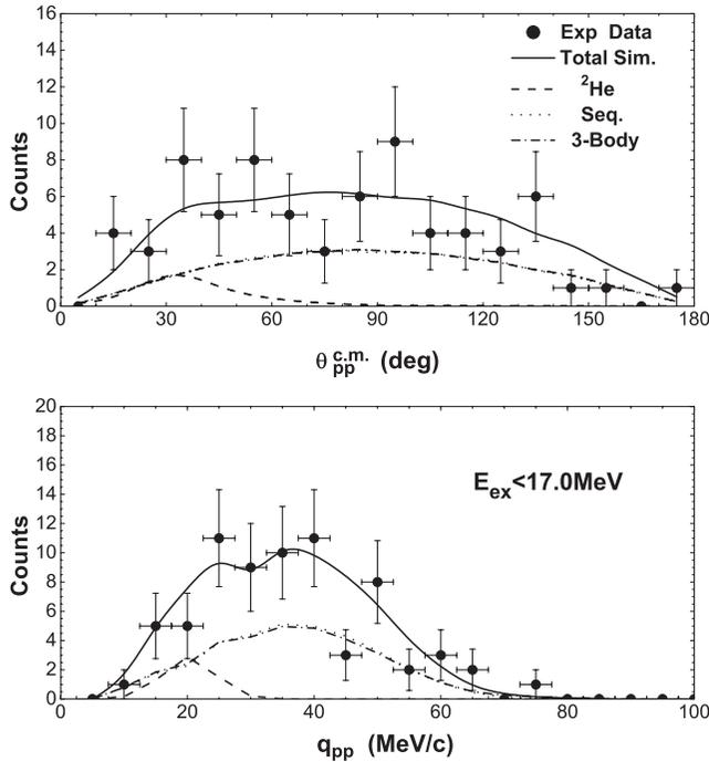
FIG. 6. Spectrum of the opening angle (top) and the relative momentum (bottom) of the two protons emitted from excited levels of  $^{28}\text{P}$  less than 17.0 MeV, which shows two-body sequential emission or three-body simultaneous decay in phase space for the odd- $Z$  nucleus  $^{28}\text{P}$ .
