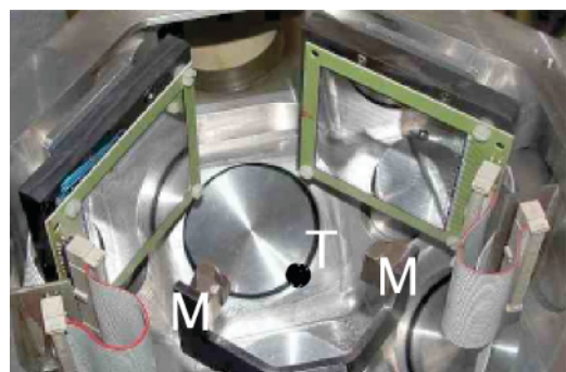
FIG. 3. (Color online) View of the telescopes pointing at the target (T) indicated by a bullet. The two magnets (M), placed on the magnetic arm, are used to deflect electrons of up to 10 \text{ keV} away from the detectors.
