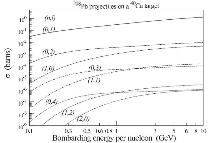
FIG. 2. Excitation cross sections for various  $(n, \ell)$  levels of the GDR in  $^{40}\text{Ca}$ , due to Coulomb excitation by  $^{208}\text{Pb}$  projectiles. Levels with the same number of phonons are indicated by the same type of line. These calculations are done using the Goldhaber-Teller description of the GDR.
