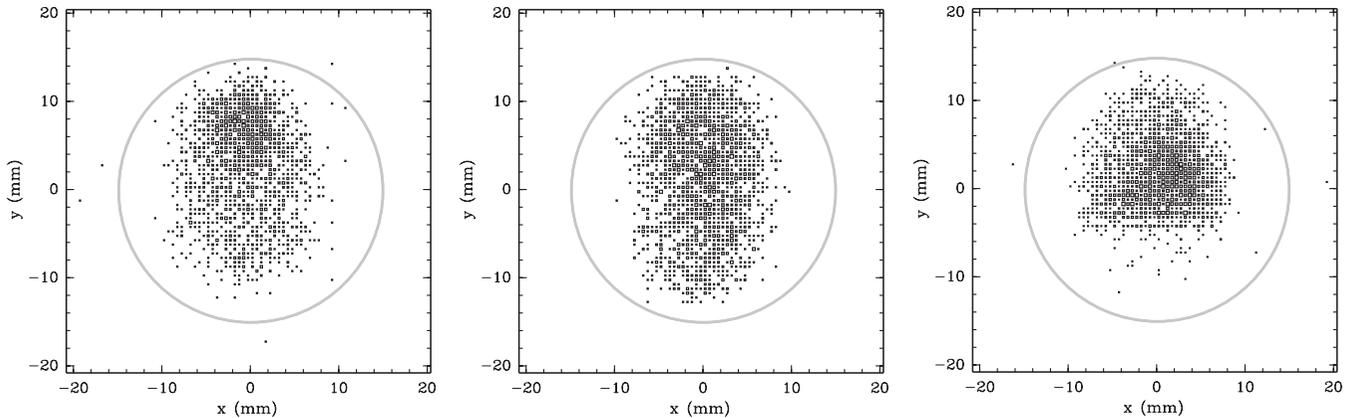
FIG. 2. The position distributions of the incident beam particles in the  $x$ - $y$  plane in the 5 GeV/ $c$  beam (left panel), 8 GeV/ $c$  beam (middle panel), and 12 GeV/ $c$  beam (right panel). The outline of the target is shown as a shaded circle.
