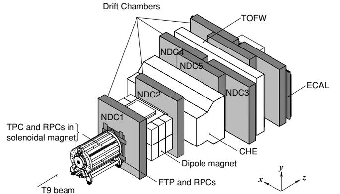
FIG. 1. Schematic layout of the HARP detector. The convention for the coordinate system is shown in the bottom-right corner. The three most downstream (unlabeled) drift chamber modules are only partly equipped with electronics and are not used for tracking. The detector covers a total length of 13.5 m along the beam axis and has a maximum width of 6.5 m perpendicular to the beam. The beam muon identifier is visible as the most downstream detector (white box).
